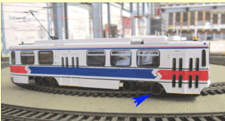
Exhibit H - Car 9111 derailed on 6 inch radius curve.
